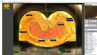
Documentation of the microsection according to DIN EN ISO 1463 by analysis software X-Scan
