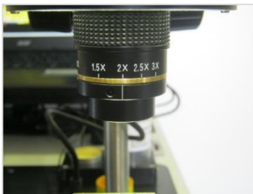
Zoom lens with snap-in function
