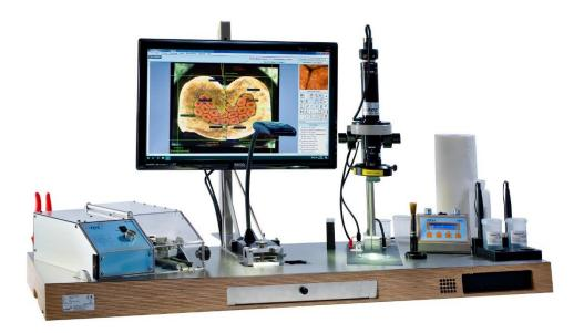
With the Microlab ML 3700-pc you can prepare microsections of crimped contacts in a very professional and comfortable manner.
