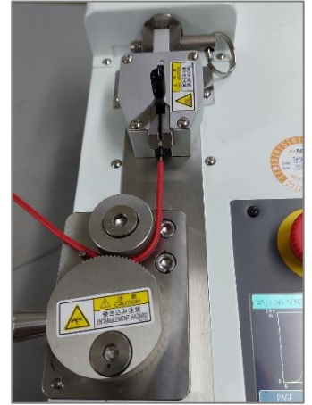
Firm fixing of the sample on the crimp and cable side
