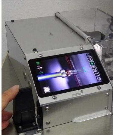
JDS Drive System incl. Visual Cut Camera (VCS)
