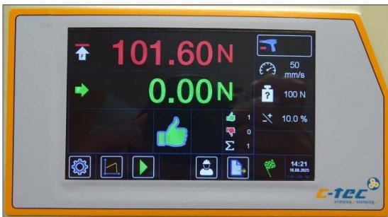
Display of the maximum force value with evaluation of the test result
