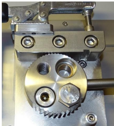
Cable tensioning system converted to fine toothting
