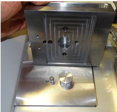
Hold the clamping crown holder at the front and back and pull it vertically upwards. The holder must be removable by hand.
