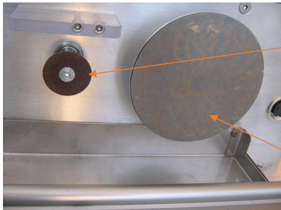
(1) Cutting disc \varnothing 24mm, inner diameter \varnothing 5mm
